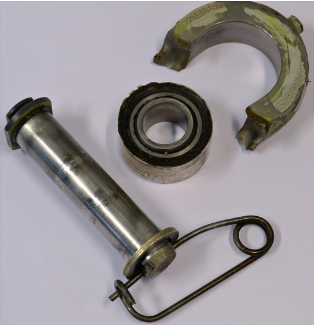
Figure 4: Upper forward suspension bar fitting. Photo: AIBN
