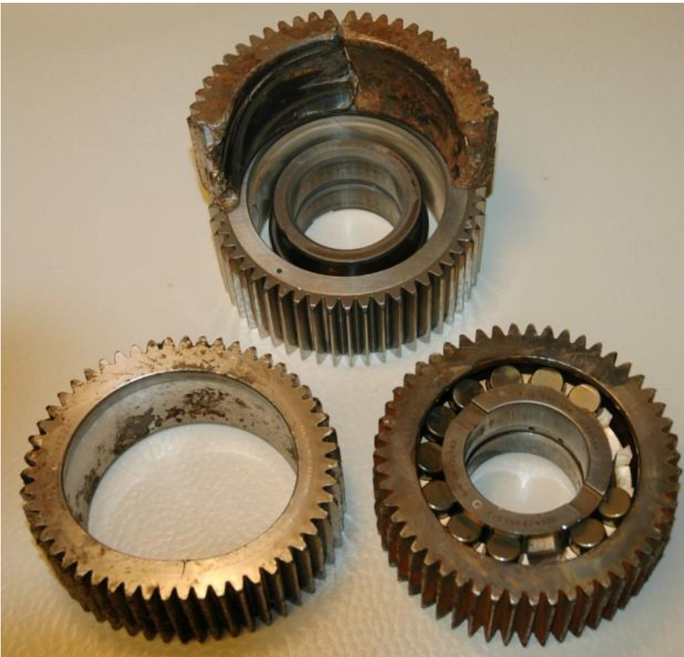
Figure 6: Parts from second stage planet gear. (The fractured gear is placed on top of a sample gear that was not involved in the accident.) Photo: AIBN
